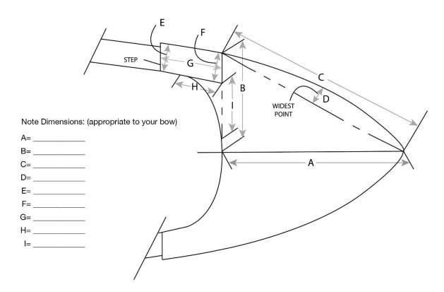
Note: if area of hatches, windlasses, etc is subtracted out, add 10% to total to account for additional material necessary to build panels.
