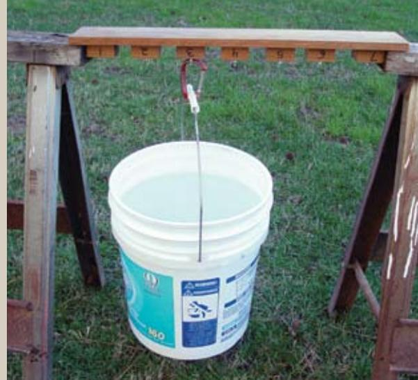
*There were no signs of seam failure during our adhesiveness test when each seam was subjected to 35 pounds of pull.*
